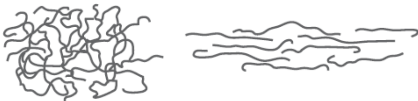
The long chain molecules in unstretched and stretched rubber
